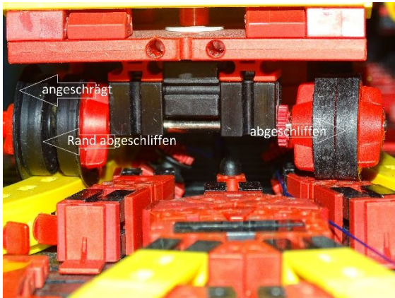
Abb. 7: Gemoddete Räder in Detailansicht
